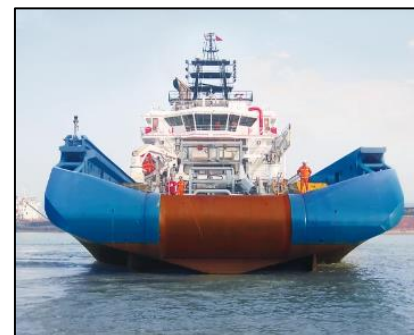
Figure 16.11-1-AHTS Stern View Showing Stern Roller
