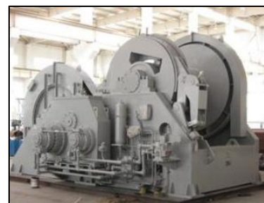
Figure 15.7-1 -Anchor handling and towing winch
